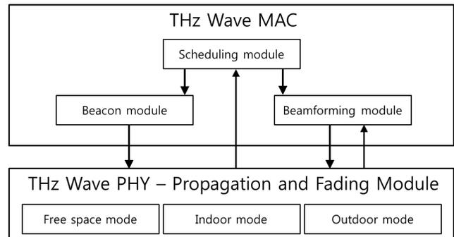
Fig. 1. THz Communications Simulator Architecture.
